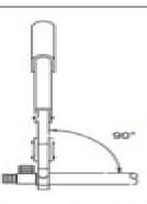
The ring must be attached straight. Center the crimping tool jaws exactly over the ring. Keep the tool at 90° and close the handles completely. DO NOT CRIMP TWICE.
