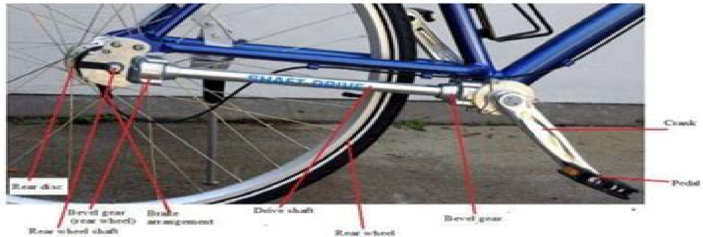
Figure 2.1- Parts of Drive Shaft
